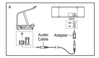
B. Plug one end of the audio cable into the jack on the side of the trainer near the power cord. Plug the other end of the cable into the LINE OUT jack on your stereo.
